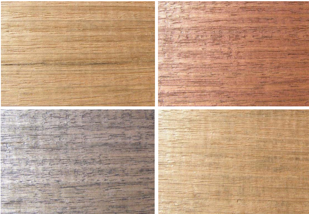
The effect of coatings and stains on wood affected by sapstain.
